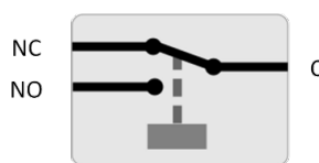
Relay configuration (not energised).
