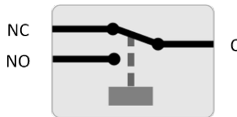
Internal operation of the programmable relay
