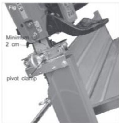
Fig 4a. Position the chainsaw bar guard around the top rod of the pivot clamp. Securely tighten the bar guard with bolt and nut provided
