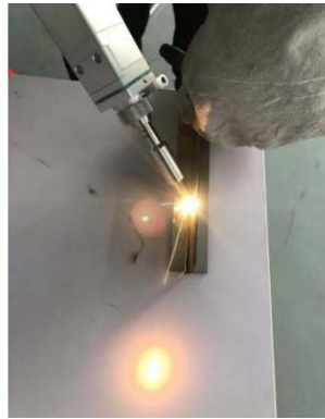
Internal corner welding diagram
