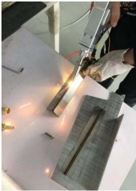
External corner welding diagram
