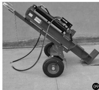
9. Put the bolt back at right position, now the main body is fixed on the draw pole
