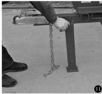
11. Keep the machine level by hand and assemble the front jack
