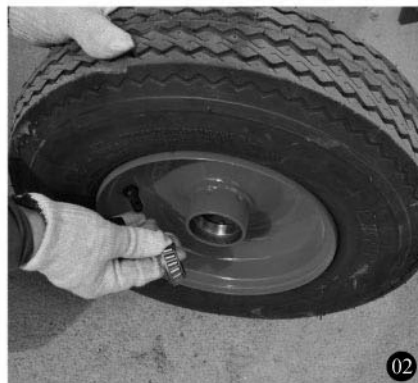
2. Assemble the bearing on each one wheel
