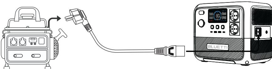
**⚠** For stable and efficient charging, avoid using unreliable power sources like wind turbines. Also, it's not recommended to run your devices with AC70P while it's charging with a generator.
